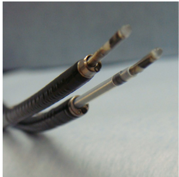
Figure 2: A 3.0-mm ultrathin bronchoscope with a 1.4-mm ultrasonic probe (left), and a 4.0-mm bronchoscope with a 1.95-mm guide sheath and a 1.4-mm ultrasonic probe (right).
